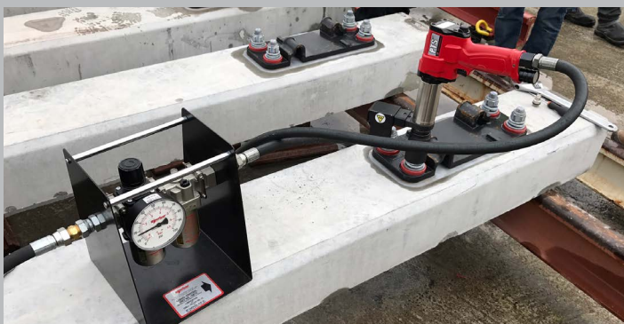
Norbar PneuTorque® PTS-52-500 multiplier with Lubro Control Unit
